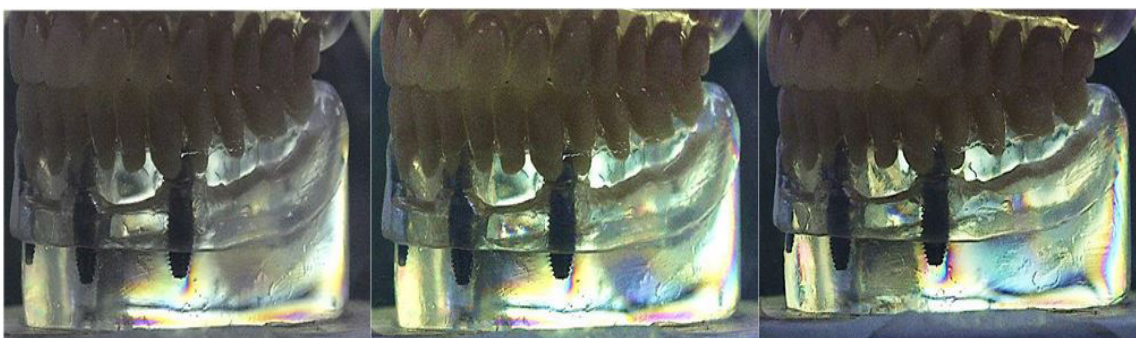
Figure 3: Left side view of the photoelastic model with three implants submitted to occlusal load (10, 20 and 30 kgf, respectively).
