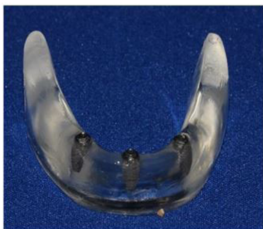
Figure 1:: Mandibular photoelastic model with three implants.
