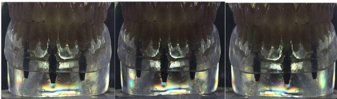
Figure 2: Anterior view of the photoelastic model with three implants submitted to occlusal load (10, 20 and 30 kgf, respectively).
